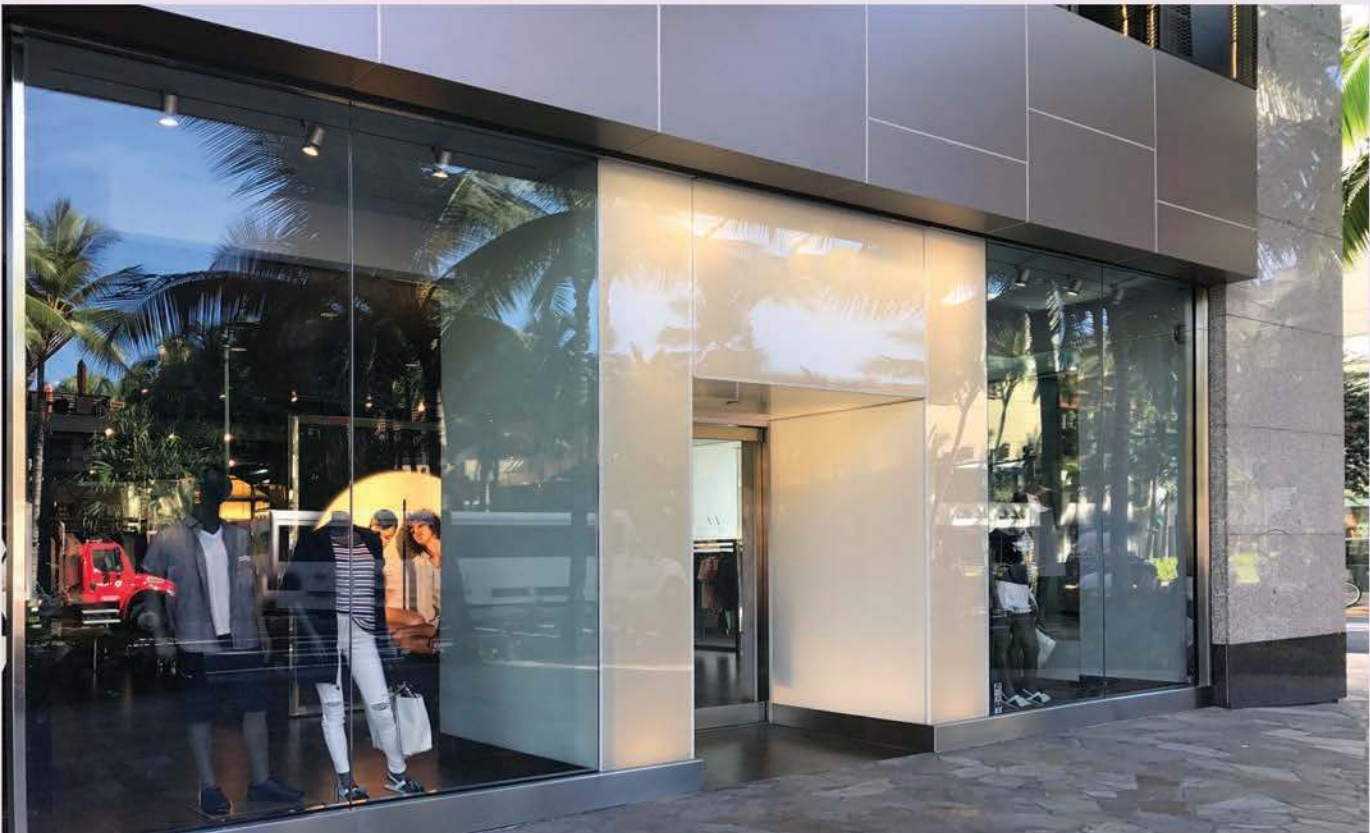
Sidelites with PL-600 Dryset Sidelites Rails
